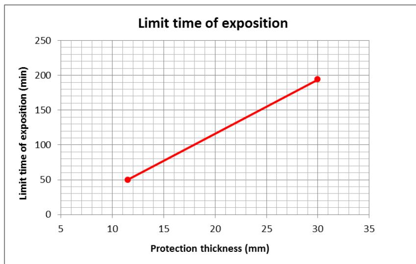
**Insulation.** The thermal insulation of the mixed slab + the protection according to EN 1363-1 is:
